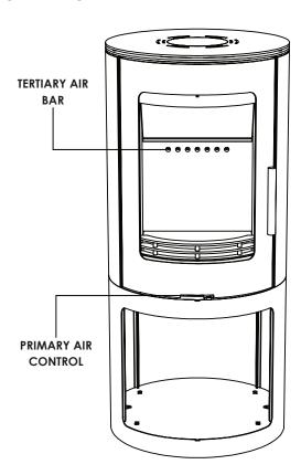
Primary Air - Slide Control - Slide right to open and left to close. Open this when you start a fire, and to regulate the stove burn. The more the stove primary air slide is open the more air is being introduced to the stove. Whilst this is useful to start a fire it should be closed significantly for the best efficiency.
