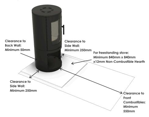
It is possible to fit the stove with less clearance around it – down to 50mm, but the non-combustible material around it must be at least 150mm thick. Take care that the wall finish is suitable to withstand temperatures of up to 200°C.
