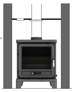
Typical Installation for Large Chamber Fireplaces - Rear Flue -Side View
