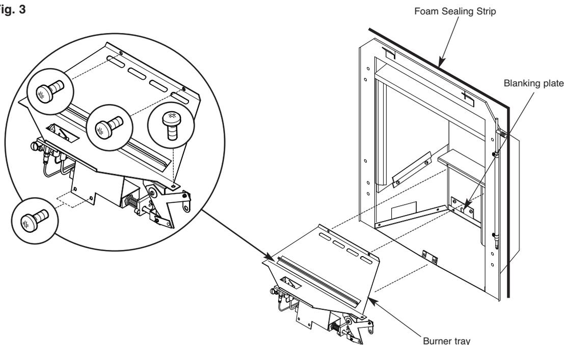
5. When the burner tray has been removed, decide which side of the appliance the gas supply will be entering the radiant box and remove the relevant blanking plate (left or right hand side). The gas supply should be concealed as much as possible.
