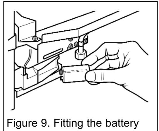
Figure 9. Fitting the battery
