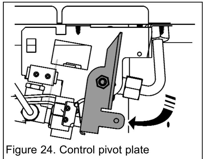
Figure 24. Control pivot plate
