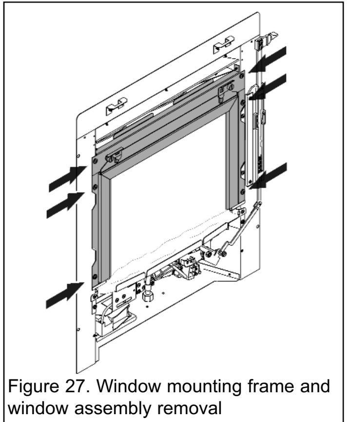
Figure 27. Window mounting frame and window assembly removal
