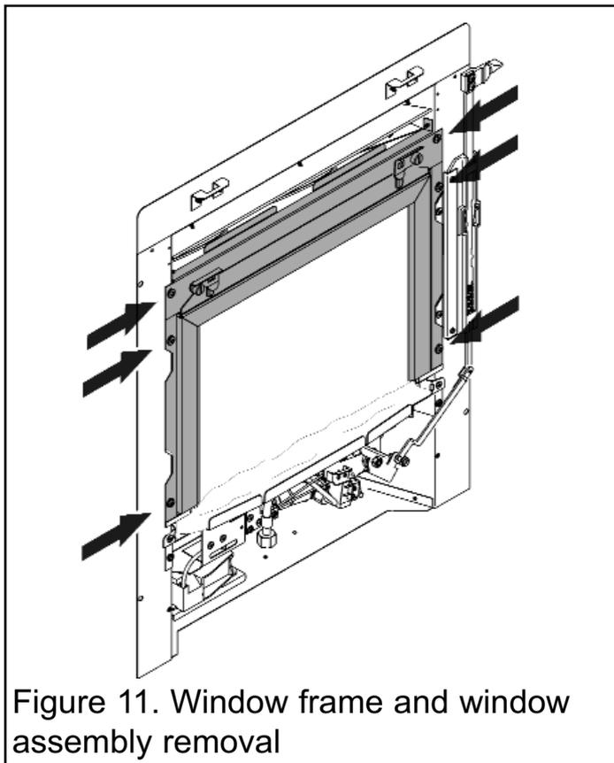
Figure 11. Window frame and window assembly removal
