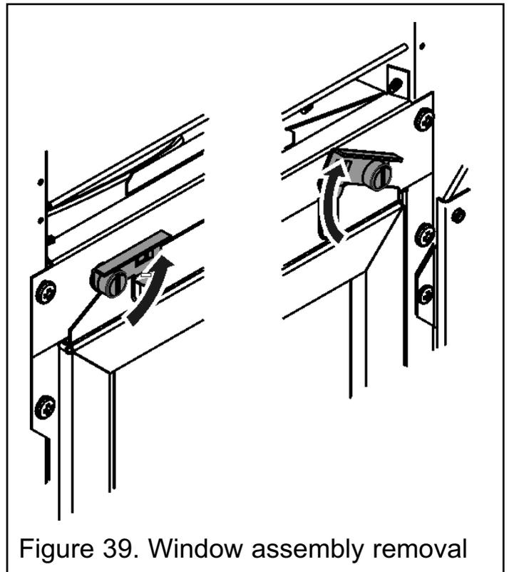
Figure 39. Window assembly removal
