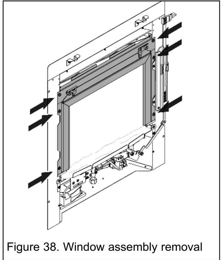
Figure 38. Window assembly removal
