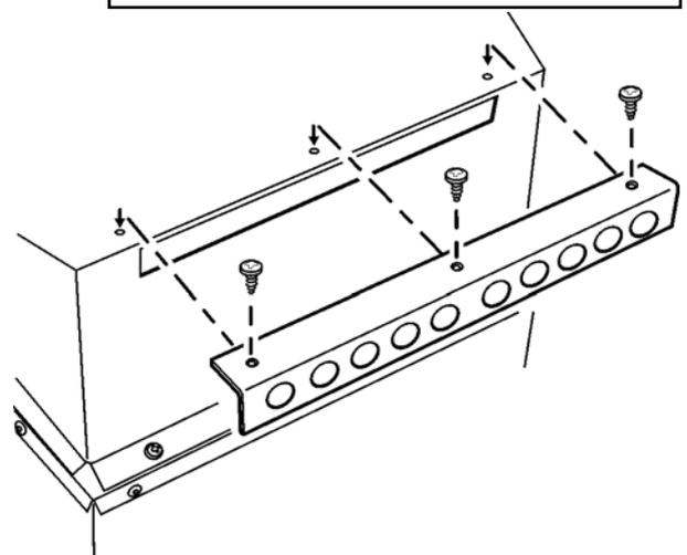
Figure 15. Flue restrictor
