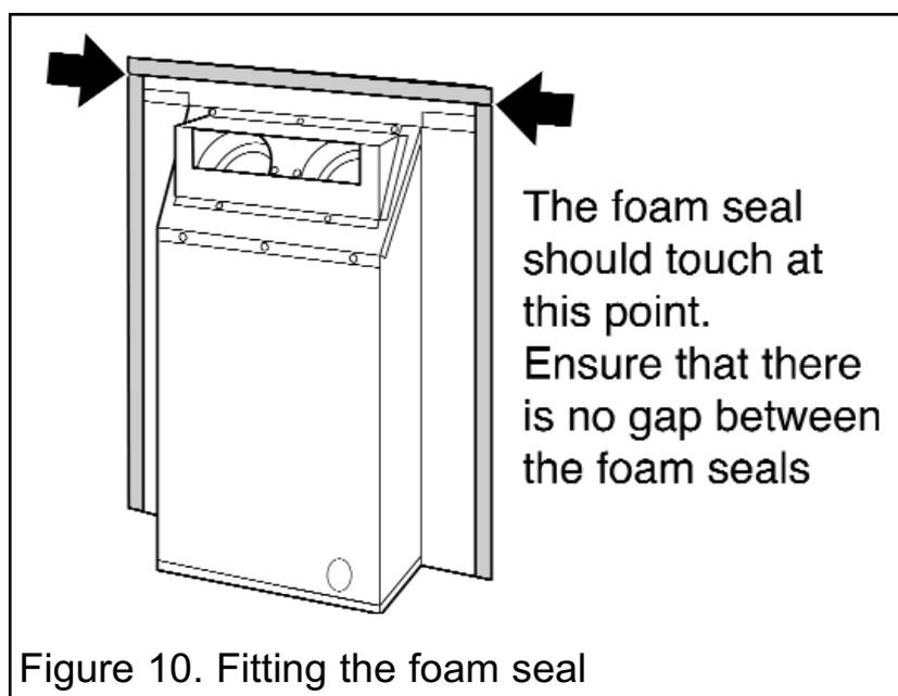
Figure 10. Fitting the foam seal
