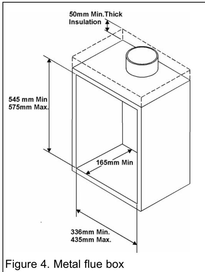
Figure 4. Metal flue box
