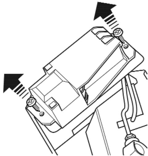
Figure 29. Removal of electronic spark generator
