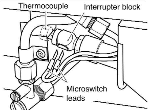
Figure 30. Thermocouple interrupter block
