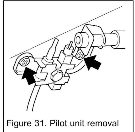
Figure 31. Pilot unit removal
