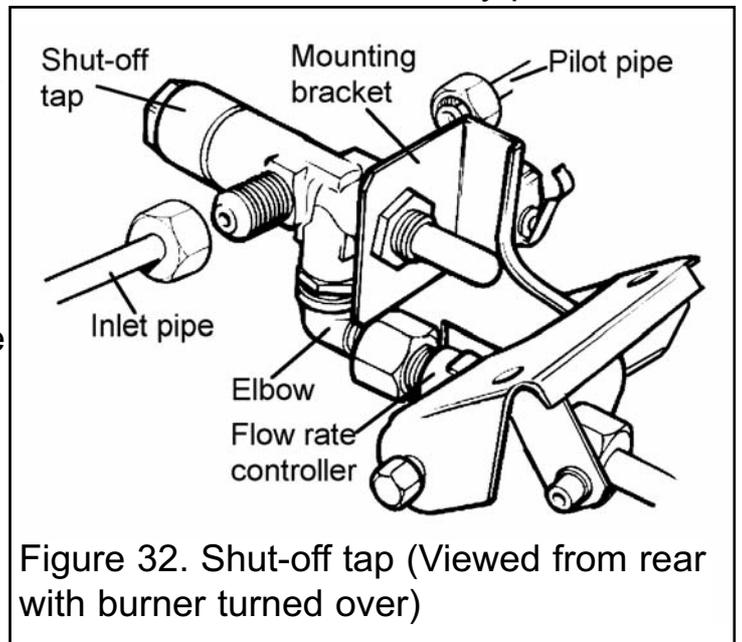
Figure 32. Shut-off tap (Viewed from rear with burner turned over)
