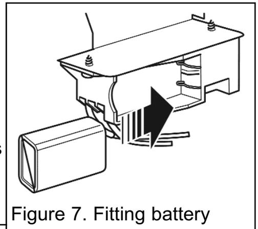
Figure 7. Fitting battery
