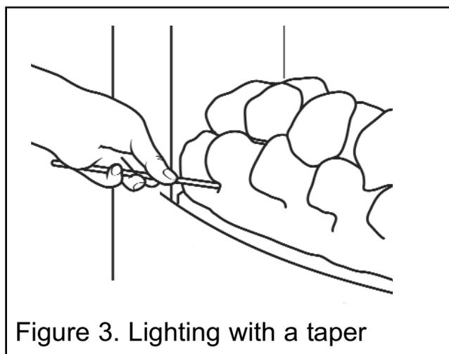
Figure 3. Lighting with a taper
