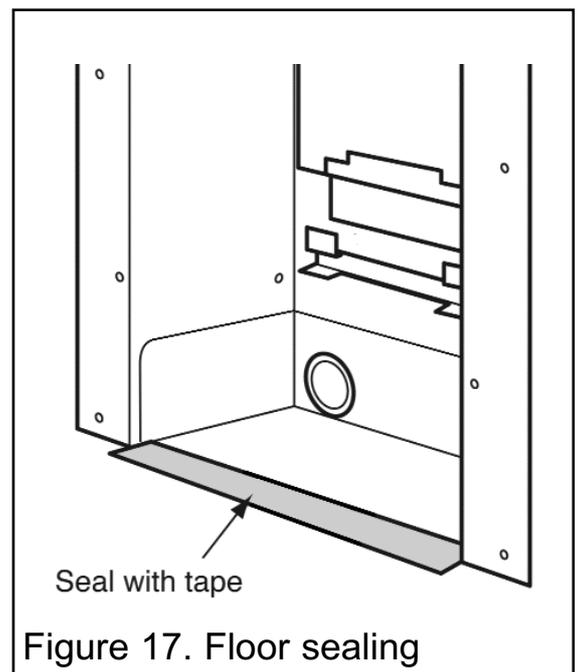
Figure 17. Floor sealing
