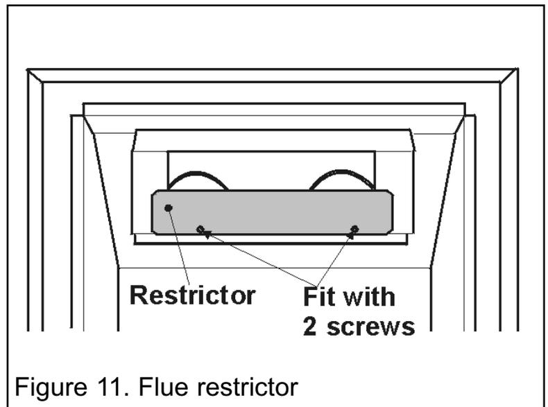
Figure 11. Flue restrictor
