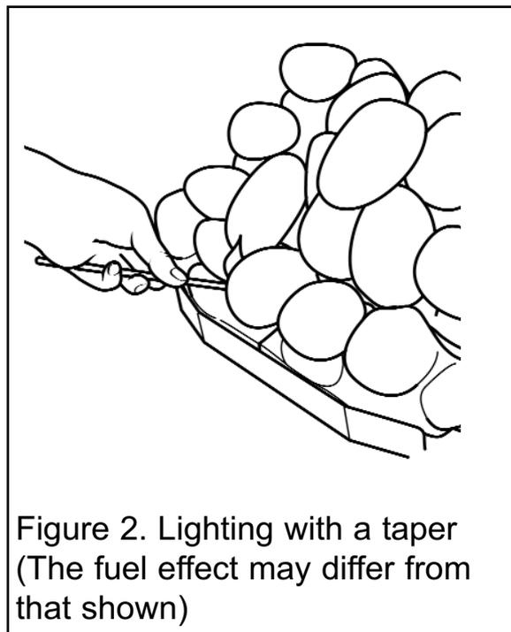
Figure 2. Lighting with a taper
