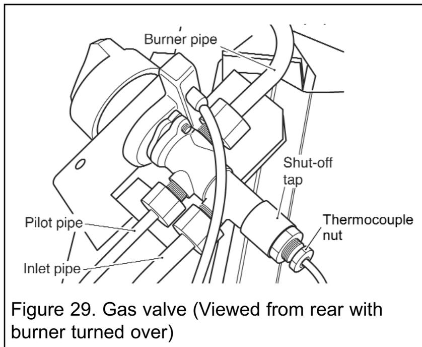
Figure 29. Gas valve (Viewed from rear with burner turned over)
