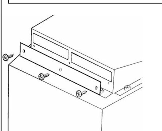
Figure 13. Flue restrictor
