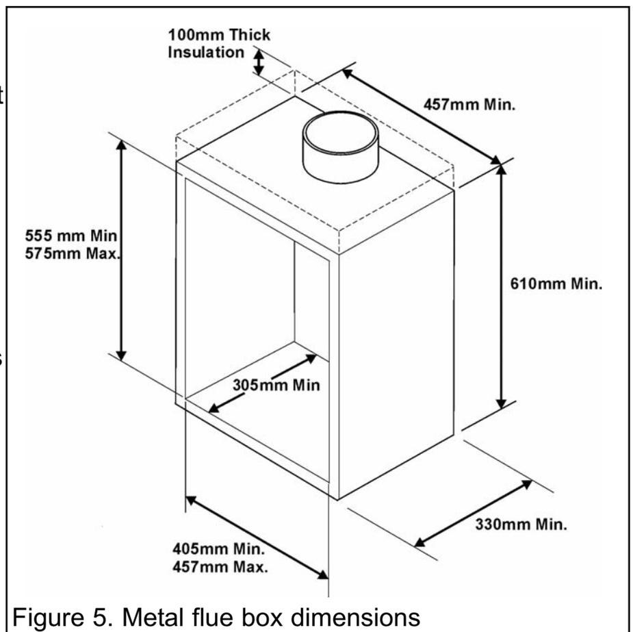
Figure 5. Metal flue box dimensions
